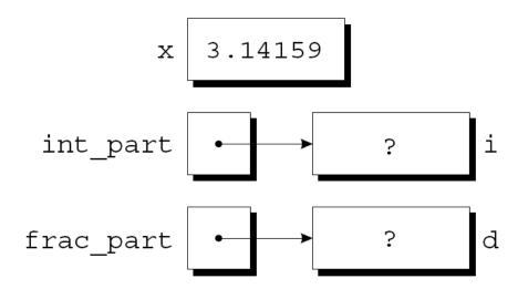
• The first assignment in the body of decompose converts the value of x to type long and stores it in the object pointed to by int part:
